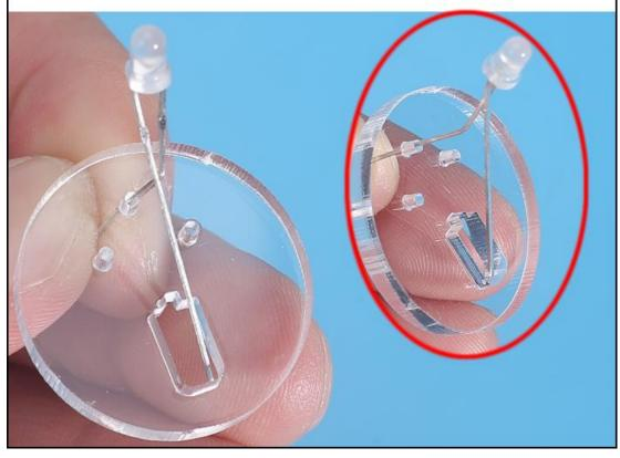
Step 25: Bend the LED to fit the LED into the largest hole.
