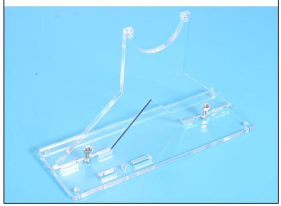
Step 12: Fix 2pcs M3+15mm Screw and 2pcs M3 Nuts and 4pcs M3 Pads on Acrylic Spring Fix Bracket.(Tips: Pads are use to connect wire and screw for Spring)
