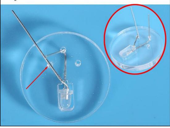
Step 27: Bend the left pin three times with pliers to make the shape shown in the picture.
