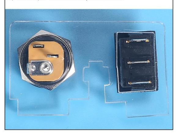
Step 20: Connect positive pole from DC-005 Power Socket and Power Switch by 10cm red Wire. Take care to select the correct pins.
