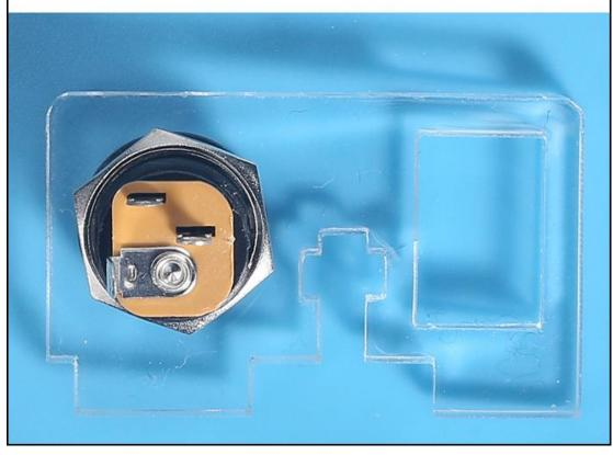
Step 19: Install 1pcs Power Switch on Acrylic Switch Bracket.
