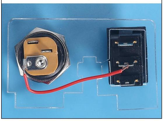
Step 21: Connect red wire form motor and pad to switch. Connect black wire form motor and pad to DC-005 Power Socket.
